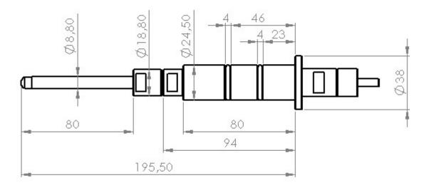
Figure 4: Drawing of the filtration probe short version
