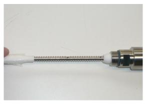
Figure 6: Mount the polypropylene membrane
