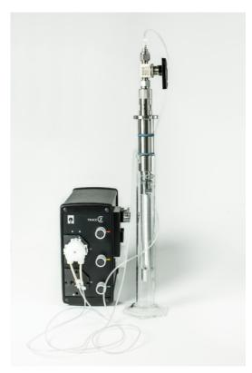
The probe is immersed into the hydrophilization solution inside an upright cylinder of sufficient length that the membrane is entirely surrounded by liquid.
