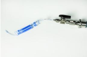
Figure 10 and 11: Connection of the filtration probe to the tubing set
