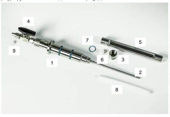
Figure 2: Parts of the filtration probe for the installation in a 25 mm side port
