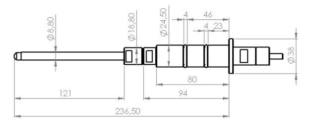
Figure 3: Drawing of the filtration probe standard version
