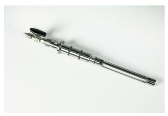
The filtration probe is sterilized together with the bioreactor and installed in a 25 mm side port of the bioreactor.
