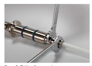
Figure 8: Tighten the cap nut
