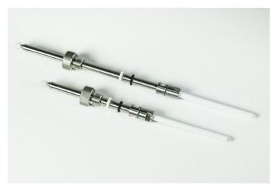
The filtration probe is sterilized together with the bioreactor and installed in a 12 mm top port with PG 13.5 thread or in a 19 mm top port using a 19/12 mm reducing adapter.
