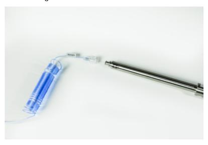
Figure 14: Connection of the filtration probe to the tubing set
