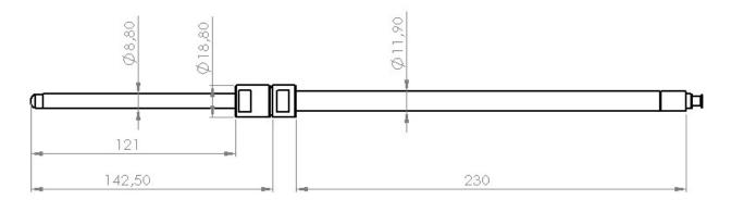
Figure 5: Drawing of the filtration probe with extension 100 mm
