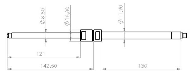
Figure 4: Drawing of the filtration probe standard version
