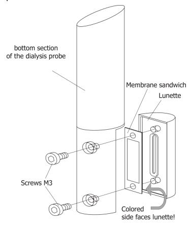
$Figure \ 10: \ Replacing \ the \ membrane \ in \ the \ dialysis \ probe \ for \ the \ application \ Glucose/Lactate$
