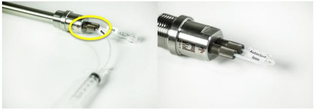
Figure 15: Filling the dialysis probe with buffer solution Figure 16: Sealing the probe prior to sterilization
