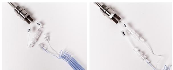
Figure 17: Connecting the dialysis probe to the dialysis tubing set
