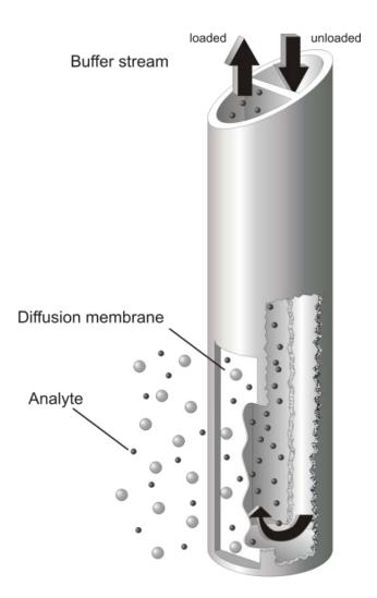
Figure 2: Principal function of the dialysis probe
