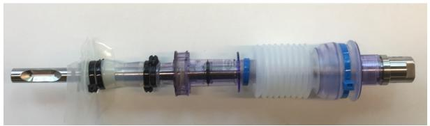
Figure 8: Dialysis probe 300 mm with Kleenpak™ Adapter
