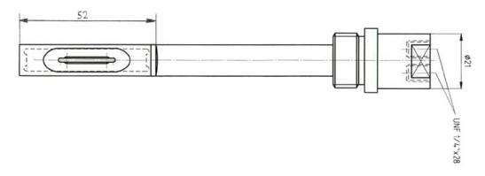
Figure 9: Drawing of the dialysis probe
