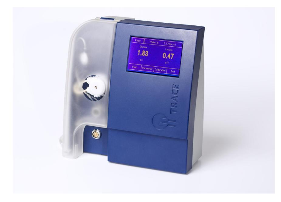
The detection is performed using a combination of an enzymatic reaction with an amperometric detection.
