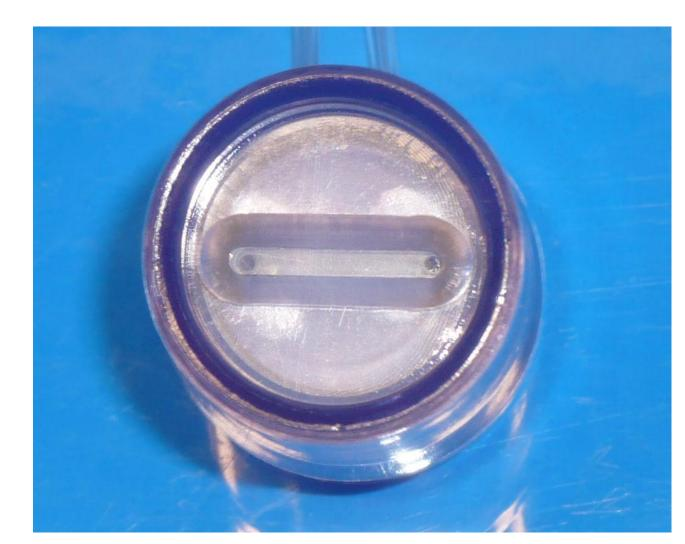
The membrane acts as a sterile barrier and is used for the separation of the analytes of interest. The dialysis plug is installed at the bottom side and sterilized together with the disposable bag.
